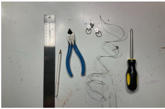
A. You will need: ruler, hanging wire, (2) D-rings (or triangle rings), (2) screws, screw driver, pencil and wire cutters.
