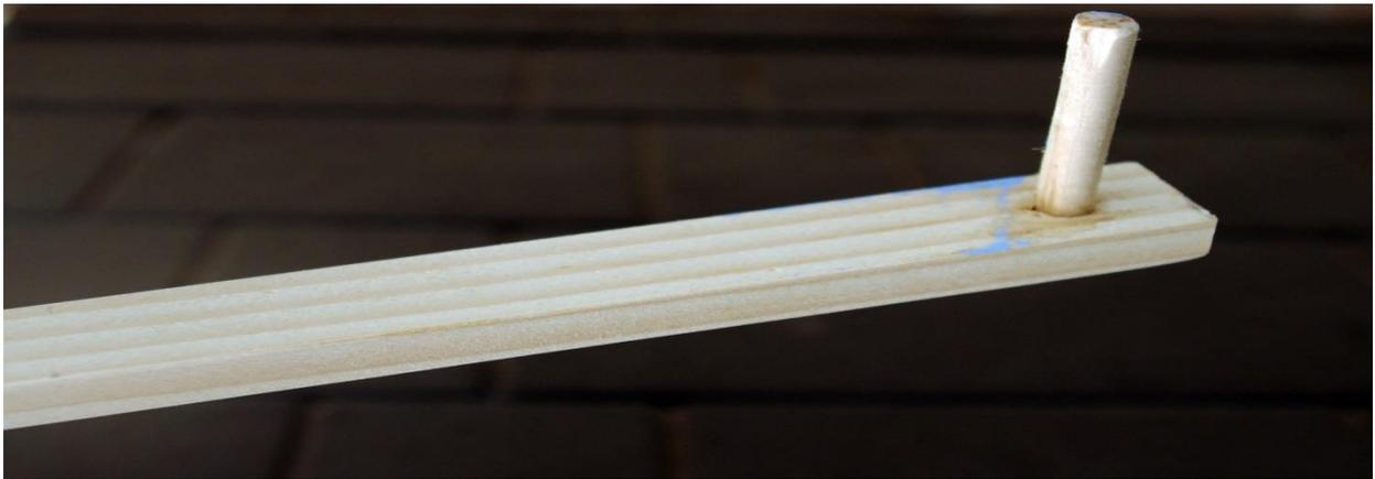
It is just a strip of wood with a peg at one end. I made mine  $\frac{1}{4}$ " x  $\frac{3}{4}$ " and the length is variable. Peg is a 2" piece of dowel. I suggest that you make a few that are six inches or so longer than the long side of the various painting supports you use. They could also be made from aluminum strip with a 2" bolt at one end.
